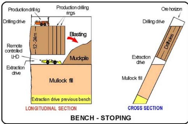
**Schematic showing bench/panel stoping mining method**
