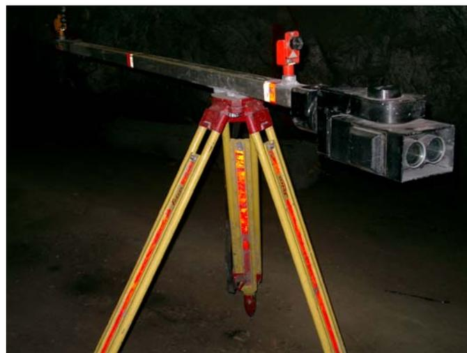
**Short Aluminium boom for tripod surveys**
