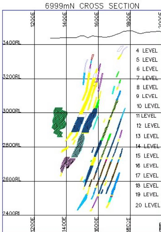
**Lead Mine X-Section showing lens type ore-bodies**
